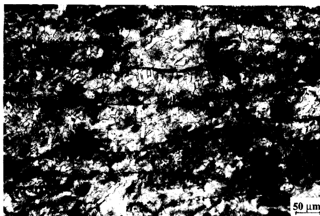
Fig. 8. Recrystallization at 20 °C after 80% rolling, Pb-2.5wt.%Sb alloy.
